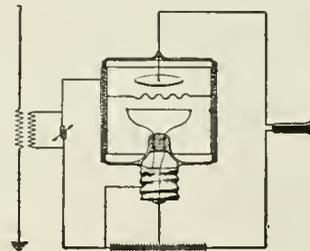
metal sleeves placed inside and outside of the tubular glass bulb. The inner sleeve supports the usual grid and is charged thru the glass dielectric from the outer sliding metal sleeve, connected in the circuit as shown.
