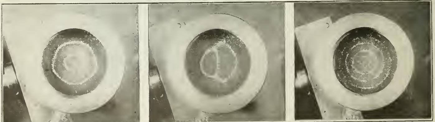
Many Valuable Studies of Sound Waves Can Be Made by Means of "Sand Figures." The Sand Is Placed on a Diaphragm Which Can Be Vibrated at Any Desired Frequency or Note.
