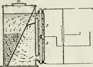
rows in diagram illustrate. The metal electrodes 7 and 8 are placed in a small chamber which communicates with the main circulating chamber thru two ports, the solution continually rising, due to heating, and passing thru the salts deposited in the lower part of the pocket formed by diagonal grid as indicated. The inventor claims that the solution will thus be kept saturated at all times and that heating is reduced to a minimum, with increased efficiency in consequence.
