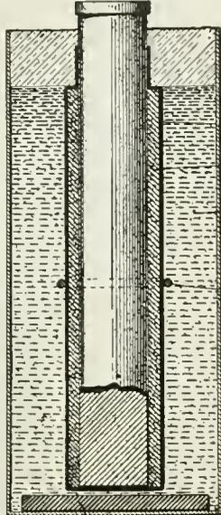
compound that long life of the cell is assured. The inventor has found that a lower oxid is desirable in combination with the higher oxid, to assure a novel and pronounced depolarizing action. He claims by this means a certain measure of transference of oxygen from the interior to the exterior of the cell, so that depolarizing efficiency does not depend merely on surface exposure, but also on the gross amount of the manganese compound.
