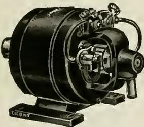
It is especially designed for lighting and charging storage batteries; will run 18 twelve volt lamps simultaneously. Can also be used as a powerful motor developing nearly 3/4 H.P. Machine is shunt wound; size 7 in. high, by 1 1/2 in. long and 6 1/2 in. wide. It is the cheapest Dynamo for its output on the market.
