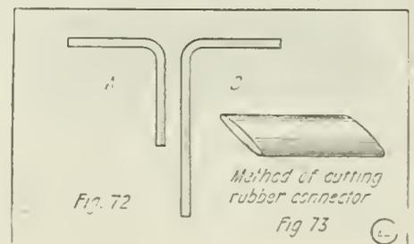
Shape of Glass Tubes Used to Connect Up the Apparatus Here Illustrated and Method of Cutting Rubber Sleeves Diagonally to Make Them Slip On Tubes Easier.
