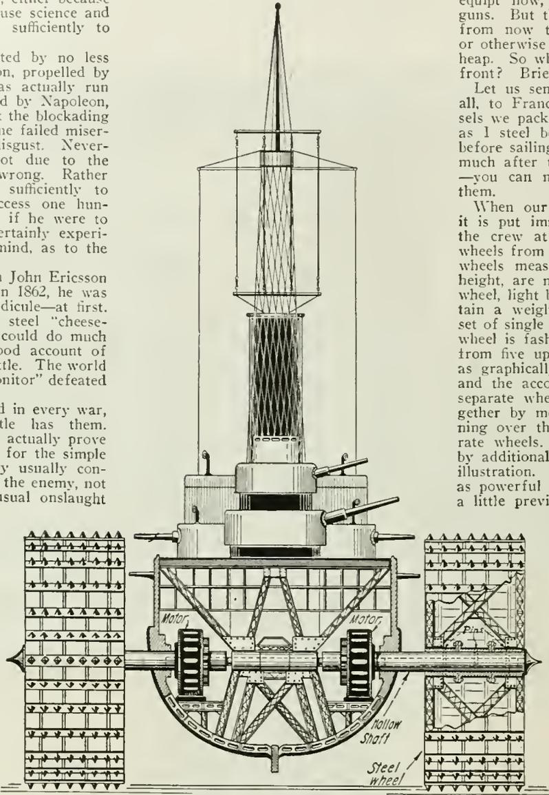
Putting Wheels on Our Battleships and How It Is Accomplished. The Wheels Here Shown Are Fashioned of Angle and I Steel Beams, on the Plan of Structural Steel Toys. Such Wheels Are Tremendously Strong. Slow Running Electric Motors Coupled to the Steel Shafts Drive the New Monster Over Land.
