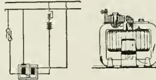
steel polarizing magnet, a set of vibrating reeds and an actuating magnet coil. The contacts on the vibrators and fixt electrodes are of special carbon to cut down arcing and sticking of contacts. By connecting the rectifying contacts in parallel a large current capacity is obtained; in series a relatively high potential current can be handled. The amplitude of movement of the vibratory contacts is small—about 10 thousandths of an inch.
