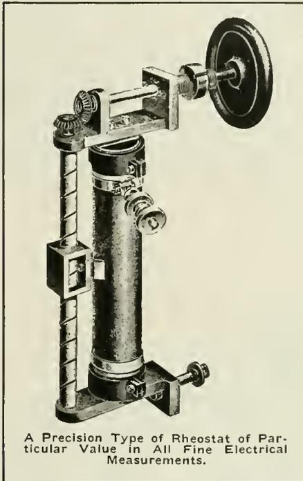
A Precision Type of Rheostat of Particular Value in All Fine Electrical Measurements.
