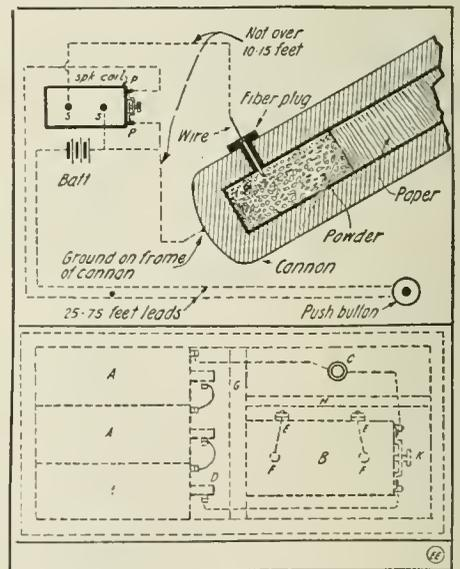
An Electric Igniter for the Toy Cannon Which Will Save Fingers, Mis-Fires and Premature Explosions.
